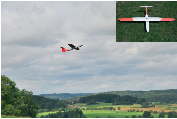
Fig. 1. Start of the unmanned aerial vehicle Carolo P200. Initially, the UAV gets manually started. Once it has reached the desired height, it can fly automatically along any predefined spline-based trajectory.
