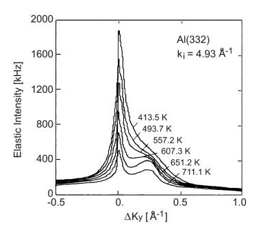
**Figure 7.** HAS angular distributions measured at around  $\Delta K_y = 0$  from the (111) terraces of Al(332) at different temperatures and with a fixed incident wave vector  $k_i = 4.93$  Å<sup>-1</sup>. With increasing temperature, an additional peak appeared which was attributed to faceting or increasing disorder (adapted from Lock et al. [47,48]).
