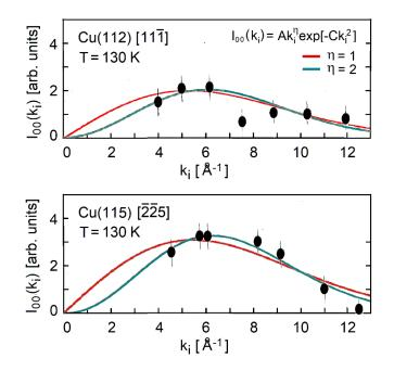
**Figure 3.** Specular HAS intensity as a function of the incident wave vector for the copper vicinal surfaces Cu(112) and Cu(115), measured at a surface temperature of 130 K along the directions normal to the steps  $[11\overline{1}]$  and  $[22\overline{5}]$ , respectively, (•, from Miret-Artés et al. [46]). Solid lines show the fits of the HAS data with Equation (6) (reproduced in the upper panel) with two different values of the exponent  $\eta$ .
