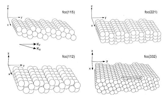
**Figure 1.** Ball models showing the structure of the (115) and (112) (**left**) and of the (221) and (332) (**right**) vicinal surfaces of a monatomic face-centered cubic (fcc) crystal (adapted from [47]). The orthogonal coordinates in the diagram are those of the vicinal surface; the wave vector component normal to steps lying in the terrace plane is here denoted as  $K_{\perp \perp}$ .
