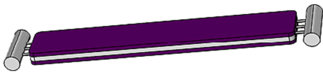
Fig. 1. Scheme of simulated reactor with the configuration of triple circular nozzles. Si substrates are displayed as violet colour and the grey one is the inner of reactor.
