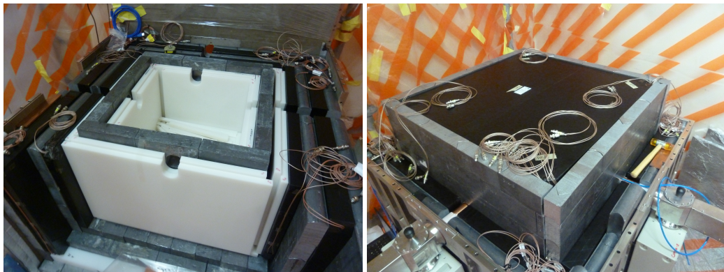
Figure 6.0.1: Left: Lower half of the CONUS+ shielding. Three out of four muon veto side layers are installed. Right: View from the closed outer muon veto.
