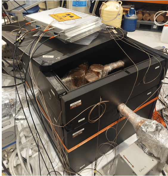
Figure 5.3.1: Muon veto test setup in LLL. The four CONUS+ detectors are installed inside the muon veto plates in the CONUS+ shield configuration.
