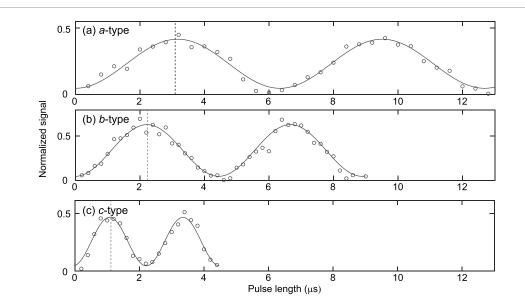
**Figure 7.** Rabi oscillation curves for (a) a-type, (b) b-type and (c) c-type transitions of the simplest triad of 1-indanol. Measured data is shown in grey open circles along with the sine fit depicted in solid lines. The  $\pi$ -pulse conditions are indicated by the vertical lines.
