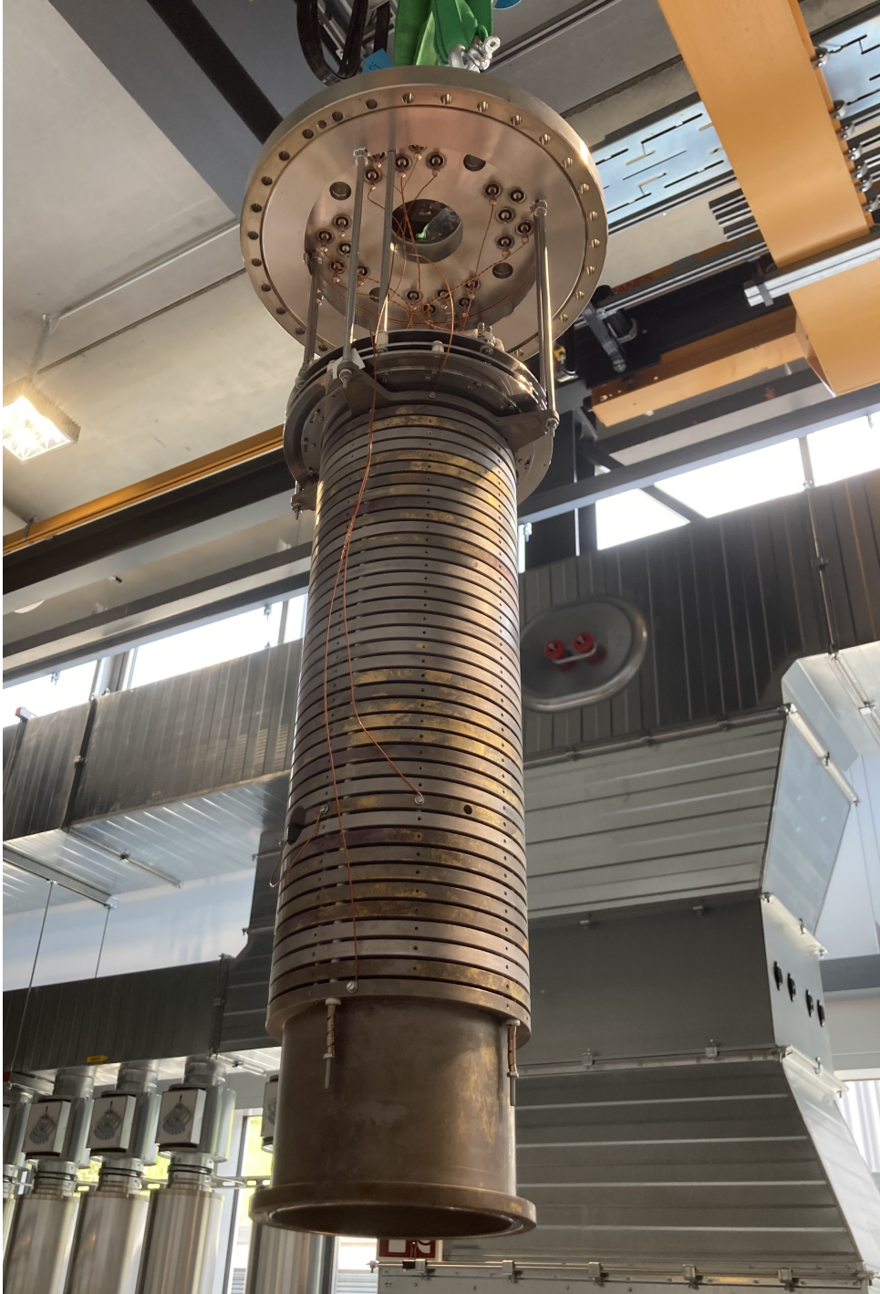
Figure 6: Image of the spectrometer in May 2023. The two visible holes in the spectrometer show the openings for the laser (small) and jet (large). The ions are accelerated to the top, the electrons to the bottom. The drift region for electrons is also seen well. Above the spectrometer, two MCPs and the delay-line-anode for ions is mounted. Copper cables are used for applying voltages and receiving signals from MCP and delay-line.
