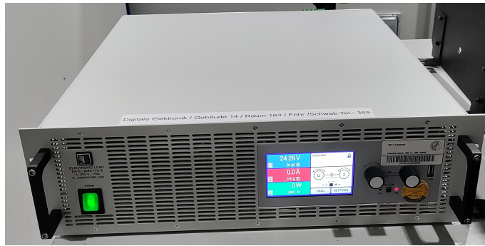
Figure 5.16: Electronic power load.
