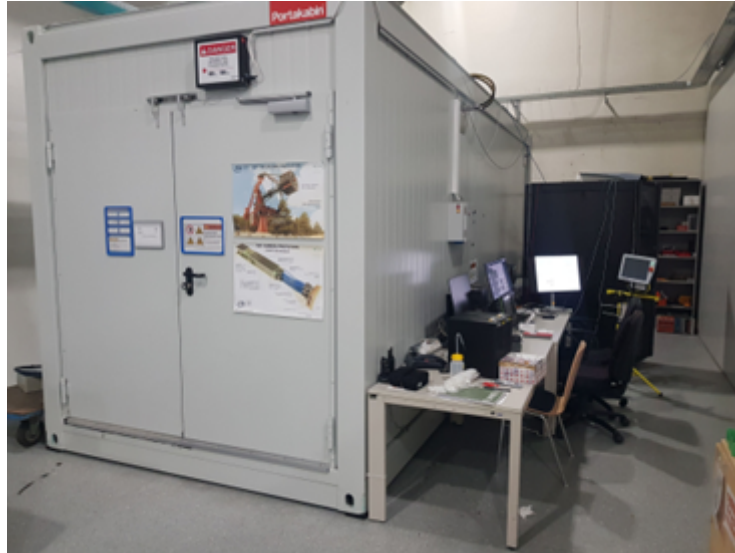
Figure 4.1: The Commissioning Facility at MPIK Laboratories: it measures approximately 6 m in length, 3 m in height and width.
