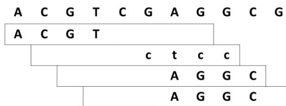
Fig. 1. Example of (8, 4) -minimizers. The shown 4-mers are the smallest 4-mers in their respective window of size 8. The second minimizer originates from the reverse complement strand and is denoted by lower letters and has to be read from right to left. The last two windows share the same minimizer, as it is often the case for subsequent windows. They are shown twice, but are only stored once
