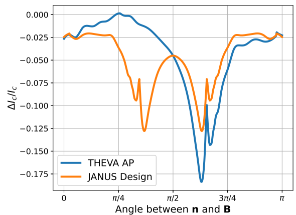
Fig. 6. I_c drop for a 5^\circ deviation in angle alignment for THEVA AP tape and JANUS design. The latter shows a much more robust angle profile with only 13% maximal I_c drop compared to 22% for non- JANUS .
