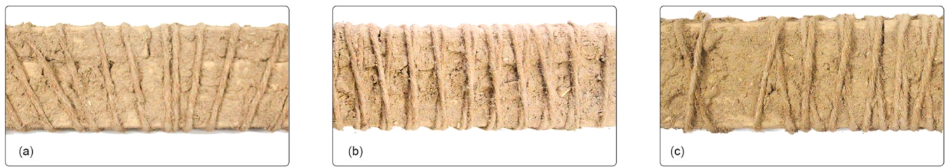
Fig. 13. Fiber wrapping pattern prototypes for four-point bending tests. (a) Tension stress line-oriented fiber wrapping pattern. (b) Uniform “X” wrapping pattern. (c) Hybrid “X” pattern with tension stress informed fiber inclination.
