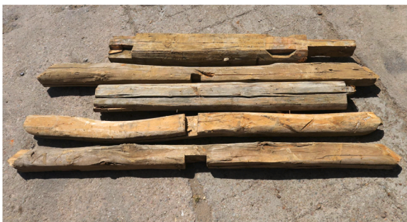
Fig. 2. Variability of cross sections and sizes among reclaimed timber pieces.
