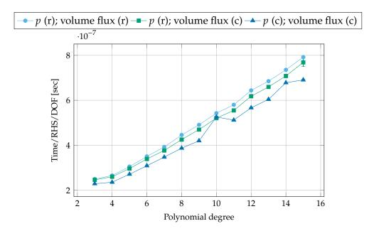
Figure 7: Influence of setting the volume flux and the polynomial degree *p* at compile time (c) or at runtime (r) on the PID of FLUXO for entropy-conservative LGL-DGSEM discretizations using the flux of Ranocha (3.10) for the compressible Euler equations.
