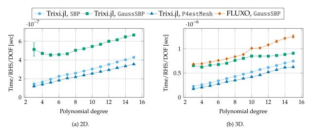
Figure 4: Runtime per right-hand side evaluation and degree of freedom for different mesh/node types and entropy-conservative DG discretizations using the flux (3.10) for the compressible Euler equations.
