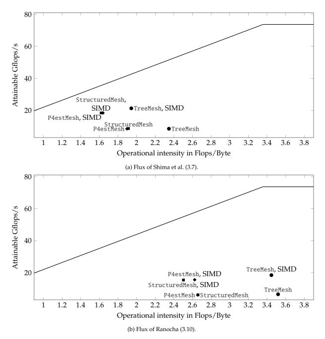
Figure 9: Empirical roofline model [74] measured using LIKWID [73] for the flux differencing volume terms of the 3D compressible Euler equations using polynomials of degree p = 3 and 8 elements per coordinate direction on an Intel® Core<sup>TM</sup> i7-8700K (CPU from 2017 with AVX2). Results are shown on the TreeMesh (circles), StructuredMesh (squares), and the P4estMesh (diamonds) of Trixi.jl.
