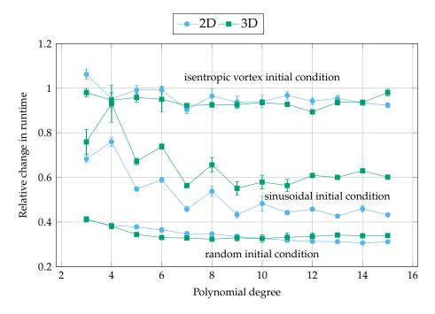
Figure 6: Relative runtime when precomputing both logarithms and primitive variables compared to precomputing only primitive variables (baseline) for flux differencing volume terms of LGL-DGSEM discretizations using the flux of Ranocha (3.10) with polynomials of degree p for the compressible Euler equations.
