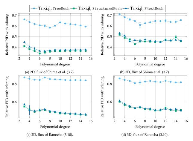
Figure 8: Relative performance obtained by inlining the volume fluxes for flux differencing volume terms of LGL-DGSEM discretizations with polynomials of degree p for the compressible Euler equations. The absolute PID with inlining is visualized in Figure 1.
