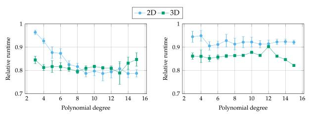
(a) Relative runtime obtained by precomputing primitive variables for the flux of Shima et al. (3.7)
