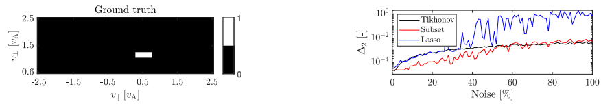
FIG. 7. The least-square subset search is superior to Tikhonov and Lasso regularization for up to around 60% noise and is able to find the exact locations of the ions generating the ICE for at least up to 10% noise in the ICE signal. The reconstructions found using 0th-order Tikhonov regularization and Lasso regularization are almost identical up to 30% noise as indicated by the almost identical value of \Delta_2 for 0-30% noise. Lasso regularization remains the worst technique for all other noise levels.
