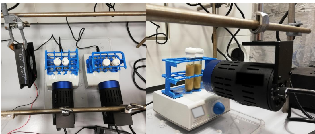
Figure S4. Experimental setup of the 440 nm photoreactor (high intensity).
