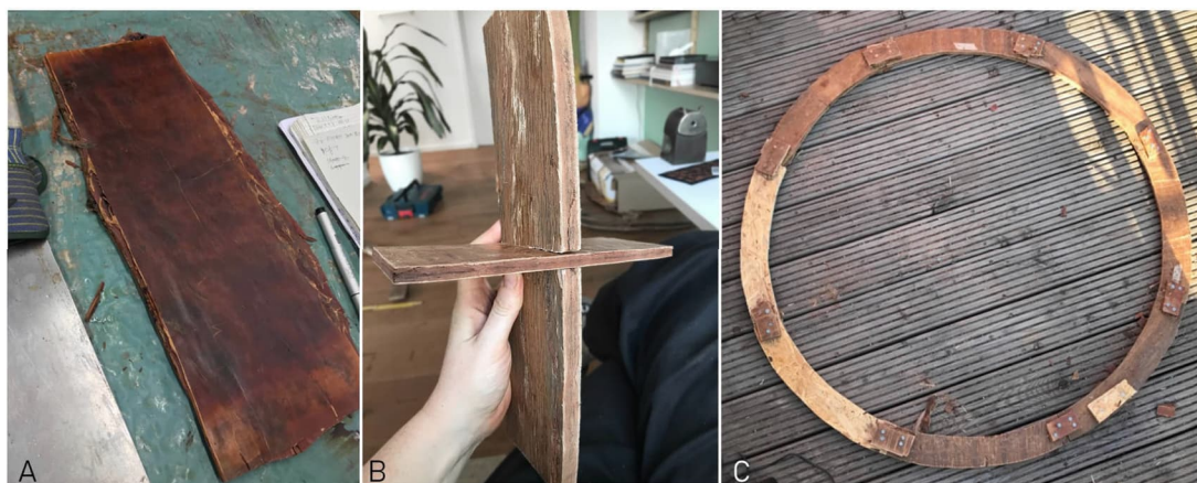
Figure 5.4.4: Fabrication test of densified bark panels. Oak, larch and spruce panels were cut and tested for the inner structure of the sphere, (A) densified spruce panels, (B) first construction test made out of densified oak bark, (C) test ring for bark sphere partly made with densified and cut bark pieces and fiber board
