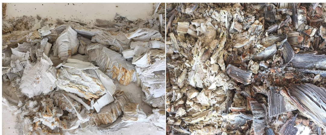
Figure 4.4. 1: Results of combustion test with bark at the University of Arts in Bremen. Left robinia bark ash, right oak bark ash with charcoal
