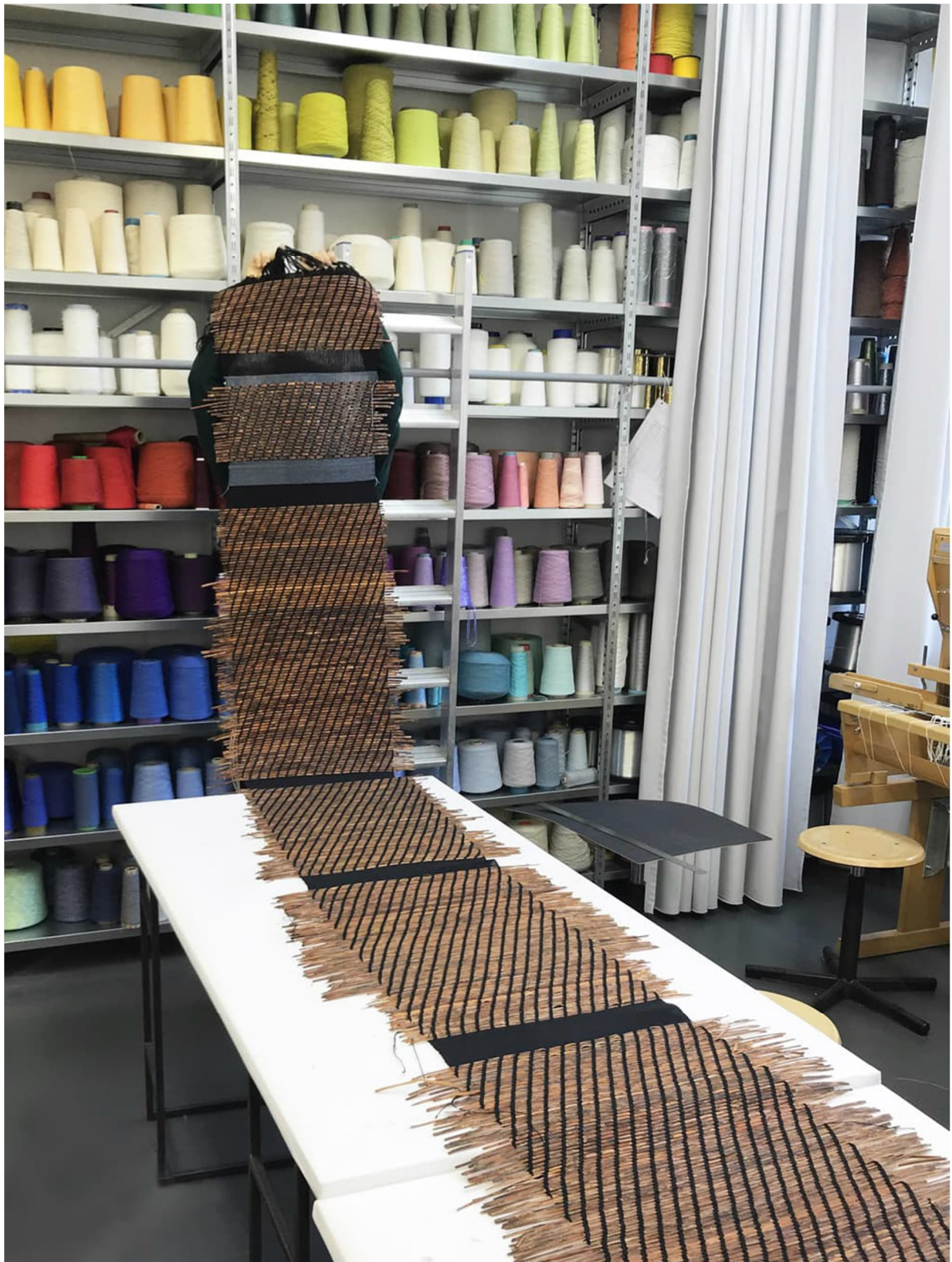
Figure 5.3.3: Woven bark section of the second jacket. 2–3mm wide, flexibilized pine bark strips were tightly woven to create a flexible and tear-resistant textile.
