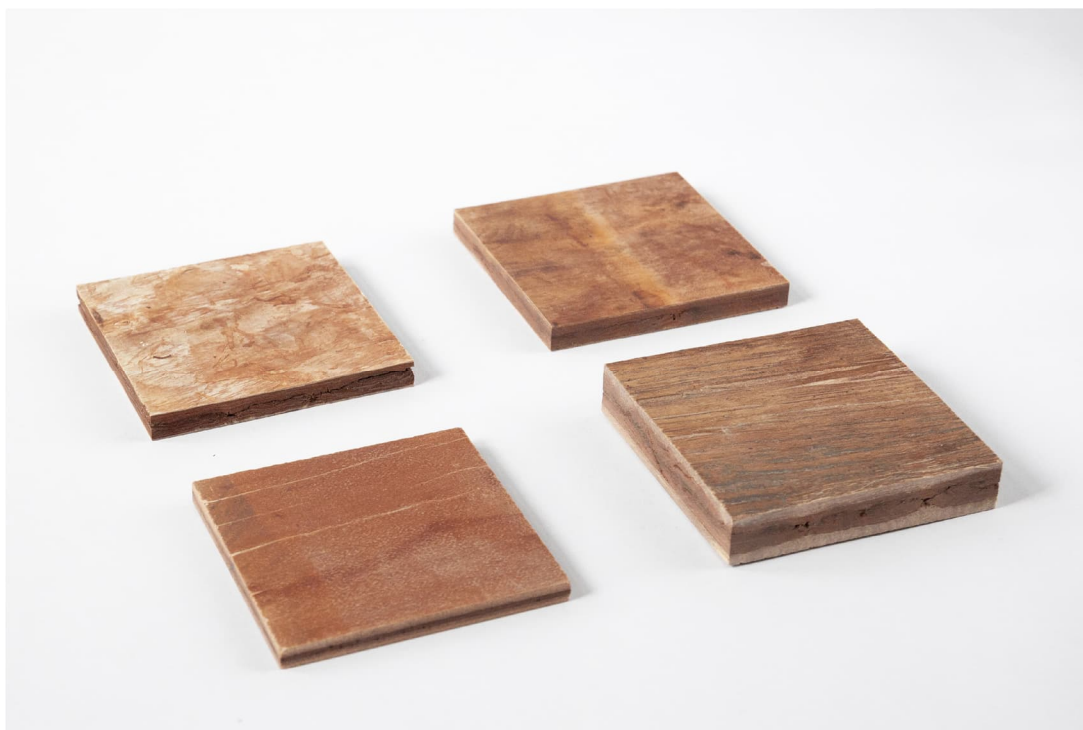
Figure 4.2.2: Bark panels made of selected bark samples. Produced panels with in-plane dimensions of 10 x 10 cm 2 showing a random thickness caused by the natural structure of the pressed bark pieces
