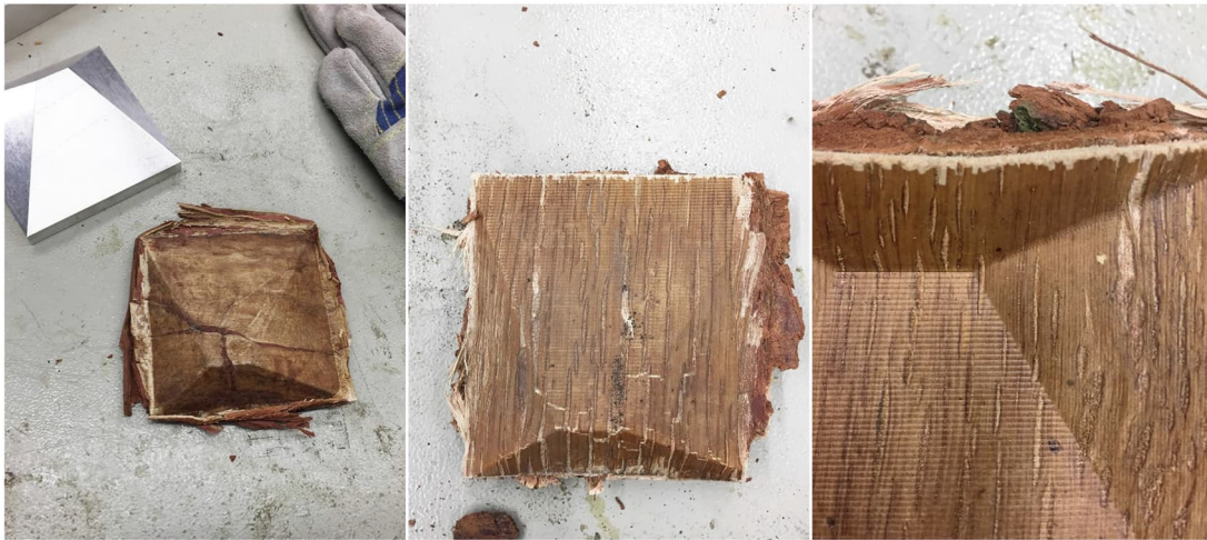
Figure 4.2.4: Larch bark and oak bark pressed in 3D form. The structure of larch bark is broken but creates a stable shape (left), oak bark can be molded into 3 dimensional shape without any major visible damages (middle and right image)
