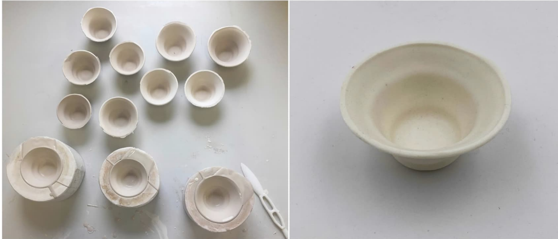
4.4.3 : Production of test bowls for glazing experiments. Left picture shows bowls just removed from the mold and bowls still drying in the mold. Right picture shows an already dried but still unfired bowl
