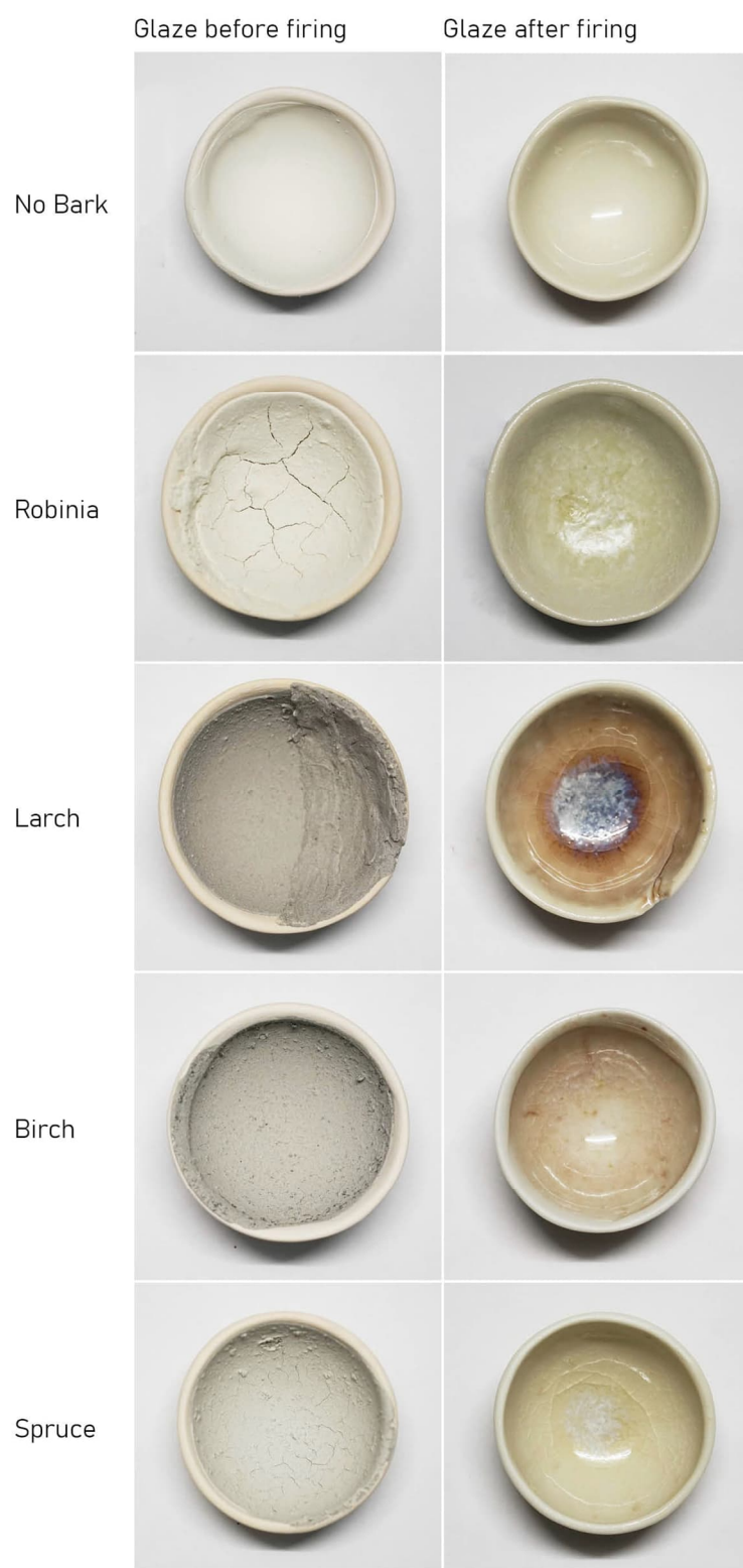
Figure 4.4.9: Glazing results of the second test with borate glaze (Tab.3.2.1). The left column shows glazed bowls before firing, the right column shows glazed bowls after firing
