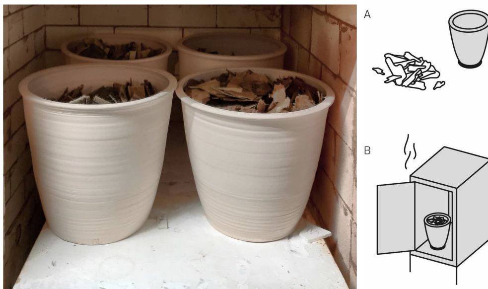
Figure 3.1.8: Production of bark ash. Furnace with bark before burning, Müritz Keramik, Close up of bark samples inside separate open burning vessels (left images), illustration shows that bark samples are placed in open vessel (A) and then fired in a gas furnace (B). Photograph taken by Müritz Keramik, Markus Böhm
