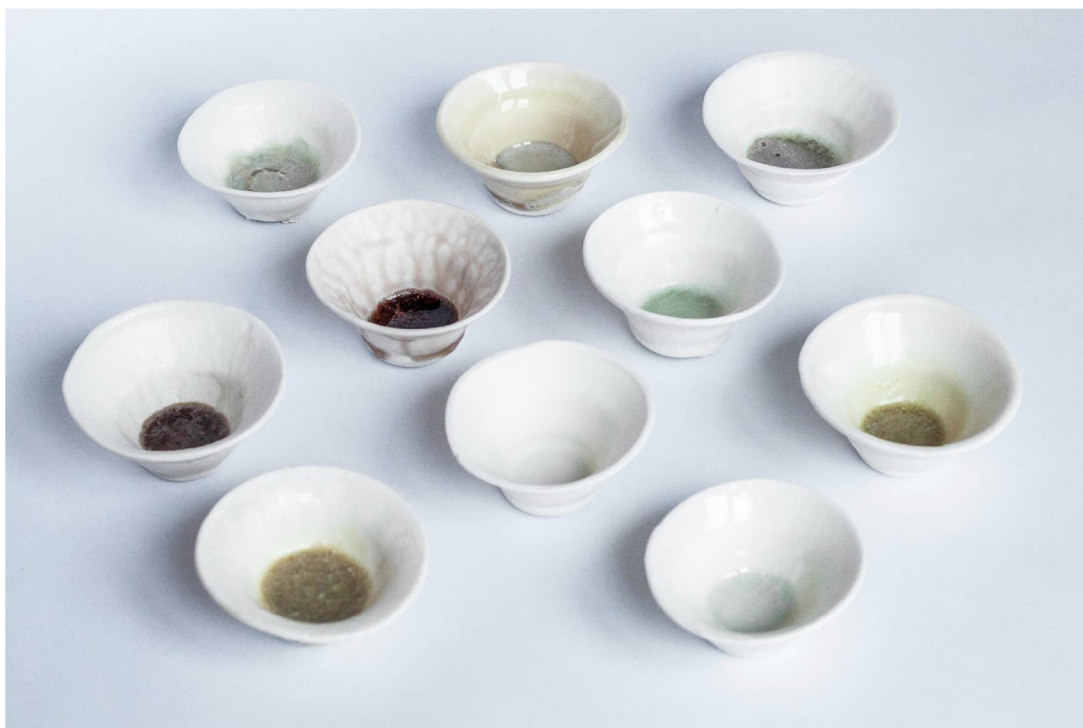
Figure 4.4.5: First glazing results with transparent porcelain glaze with borate (Tab 3.2.1)
