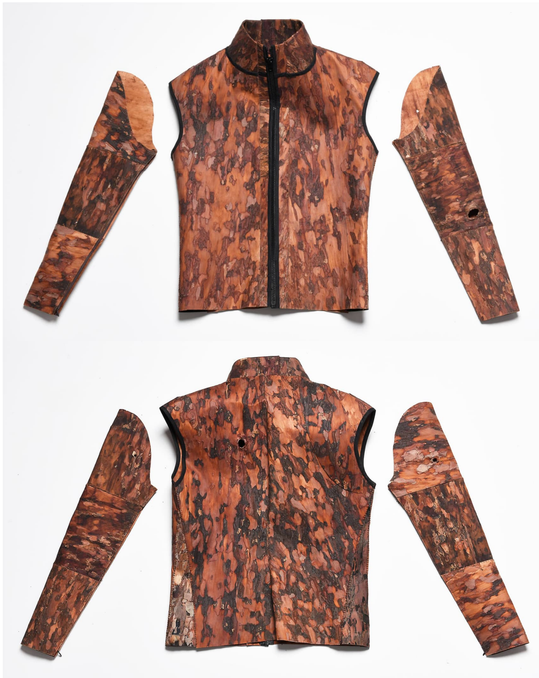
Figure 5.1.3: The production of the first bark jacket. Sleeves are made out of three pieces of bark. The vest is sewn with a leather sewing machine and lined with a ribbon. Images show the back and front of the sleeves and vest.
