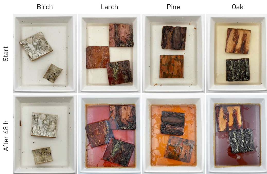
Figure 4.3.1: Bark samples in glycerol -water solution. After 48 h, a clear coloration of the solution is visible for most barks. from left to right: birch shows no optical changes, larch shows a reddish-brown dark discoloration as well as a light film on the surface of the solution, pine has a strongly orange solution with film, oak has a dark brown solution with a film.
