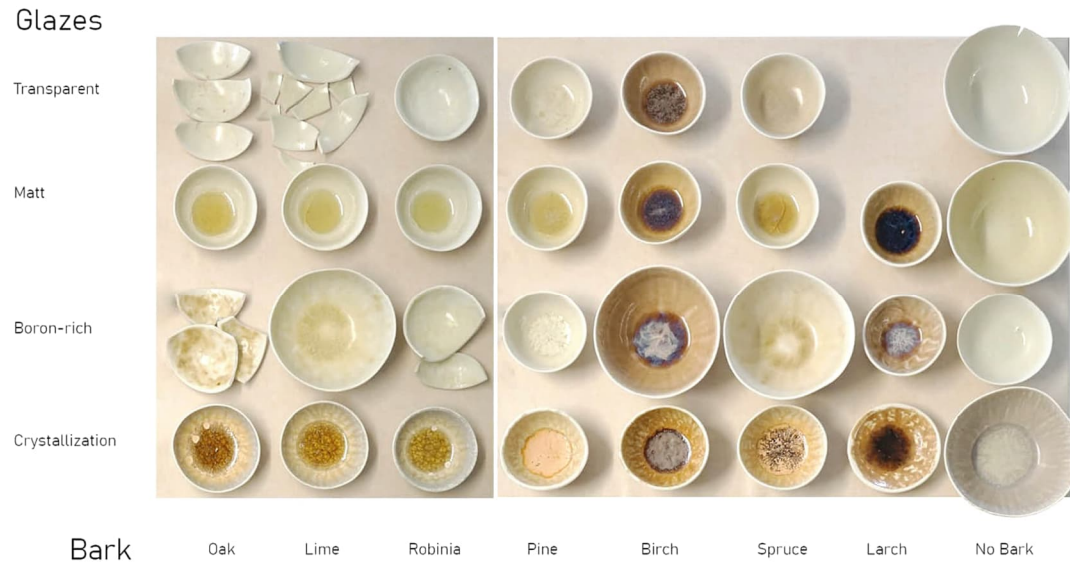
Figure 4.4.7: Overview of all bark glazed bowls after the second firing. Four different glazing recipes were mixed with bark ash and fired (Tab 3.2.1 – Tab 3.2.4)
