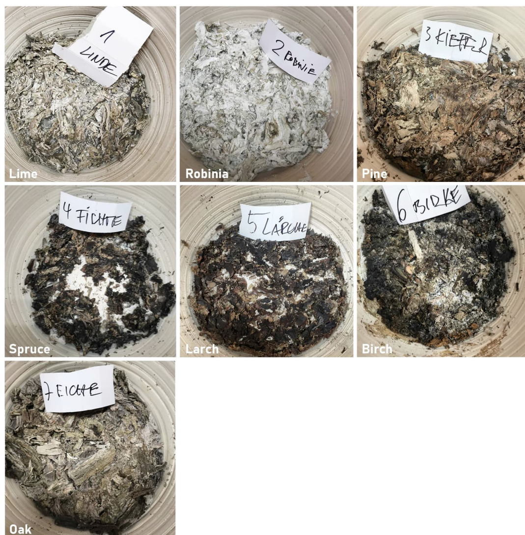
Figure 4.4.2: All bark samples after the second combustion test at "Müritzkeramik"
