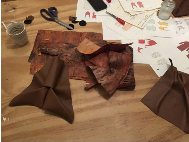
Figure 5.1.1: Design experiments for the production of the first jacket. Folding techniques were tried using leather first. Afterwards, the same folding technique was repeated in flexibilized pine bark.
