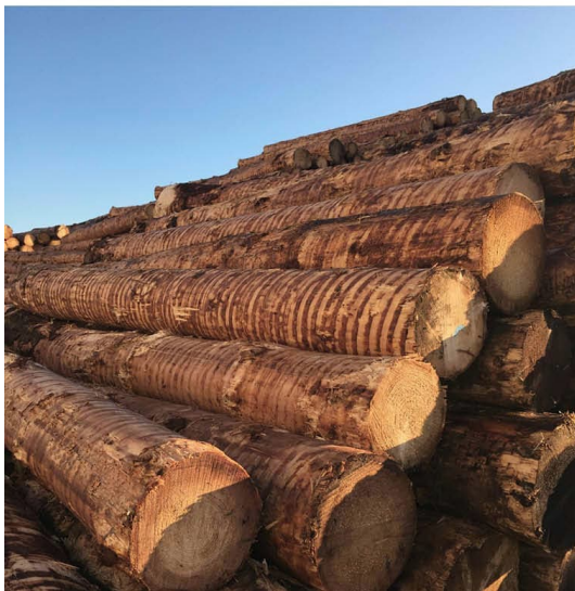
Figure 2.9: Debarked logs. Rotor debarking is the most common method of debarking in sawmill and veneer industry. Logs are driven through the machine separately and rotating blades scrape the bark along the cambium layer. The image shows debarked logs with characteristic debarking lines.
