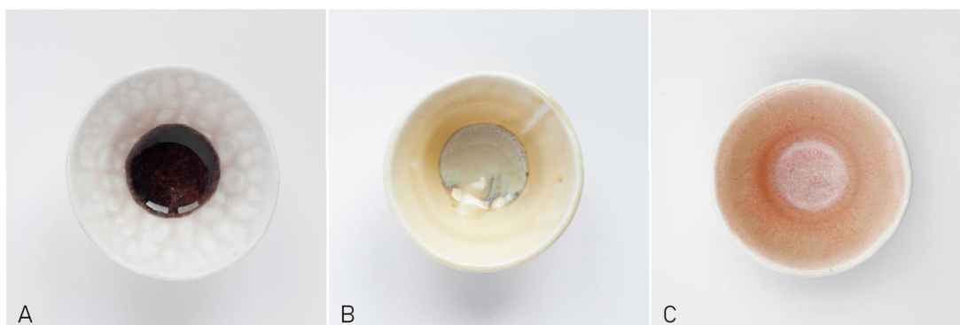
Figure 4.4.6: Selected test bowls after the first firing test (borate glaze), (A) spruce ash glaze, (B) larch ash glaze, (C) birch as glaze
