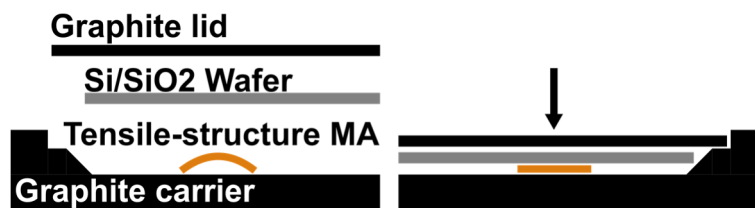
Fig. 74: Schematic illustration of the annealing assembly utilized for suppression of bending and flattening of the freestanding tensile-test structure MAs.
