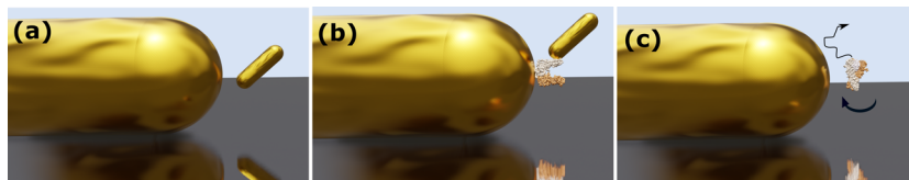
Figure 4. Few examples of optoplasmonic detection schemes based on a single sensor GNR. (a) Free small gold nanorods translationally diffusing and tumbling in the near field of the sensor GNR. (b) This detection may be even more sensitive if the diffusing nanorod is attached to a fixed position near the tip of the GNR by a biomolecule (Hsp90) and will be able to detect the conformational changes of the molecule. (c) Refractive-index-based detection of a single protein freely diffusing through the near-field zone of the sensor GNR.
