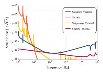
FIG. 3. aLIGO noise budget obtained from pygwinc. Only the dominant classical noise sources are plotted, along with the quantum noise. The total force noise in the system is the sum of the seismic noise and the suspension thermal noise, which is effective at low frequencies. The coating Brownian thermal noise is taken as the main constituent of the sensing noise. As can be seen from the figure, quantum noise dominates over the sensing noise by a large margin at high frequencies.
