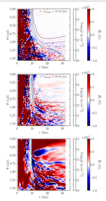
**Extended Data Fig. 5** | **Generation of the mean radial magnetic field.** Meridional profile of the mean radial magnetic field,  $B_r$ , at  $\approx$  10 ms (top), 30 ms (center), and 50 ms (bottom) for the simulation with  $\Delta x_{\text{finest}} = 12.5$  m (left column) and 200 m (right column). The rest-mass density contour curves are also plotted. The visualization is the following link
