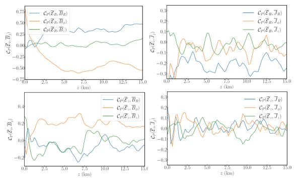
**Extended Data Fig. 7** |  $\alpha \Omega vs \alpha^2 \Omega dynamo$ . (Left) Time-averaged correlations between the poloidal electromotive force  $\bar{\mathcal{E}}_R$  (top) and  $\bar{\mathcal{E}}_z$  (bottom) and mean magnetic field components  $\bar{B}_i$  for R = 30 km. (Right) Time-averaged correlations between the poloidal electromotive force  $\bar{\mathcal{E}}_R$  (top) and  $\bar{\mathcal{E}}_z$  (bottom) and mean current components  $\bar{J}_i$  for R = 30 km.
