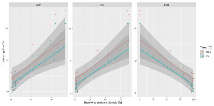
Fig. 3. Grainsize distribution and grainsize-dependence of LOI of uMlalazi samples.
