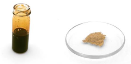
Maillard reaction products (left) and purified substituted pyrazines (right)
