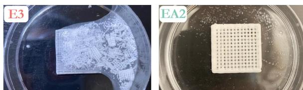
**Figure 6.11:** Emulsion inks based only on CNC/ $\alpha$ -CD (E1-E3) disintegrate in a calcium bath, while alginate-filled emulsions EA1-EA3 cross-link and retain their shape.
