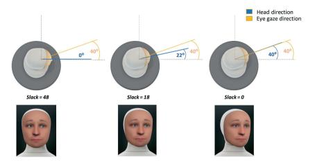
Figure 2.4: An example showing the differences in eye and head movements when looking at a target depending on the slack values.
