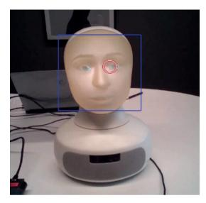
Figure 3.2: Example of Gaze Aversion detection using the algorithm. Here the gaze point (x, y) (the red circle) lies within the face's bounding box [X, Y, H, W] (blue rectangle), so it is not a Gaze Aversion
