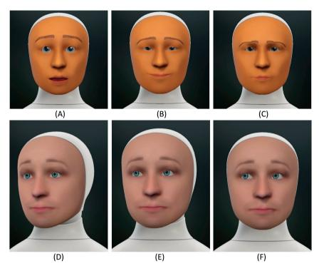
Figure 1.2: A few examples showcasing the capabilities of the Furhat robot. Subfigures (A)-(C) depict 3 facial expressions; Surprise (A), Happy (B), and Angry (C). Sub-figures (D)-(F) show 3 examples of independent eye-head movements of Furhat; both eyes and head directed at a target (D), eyes fully directed at the target but head directed halfway (E), and only eyes directed at the target with no head movement (F)
