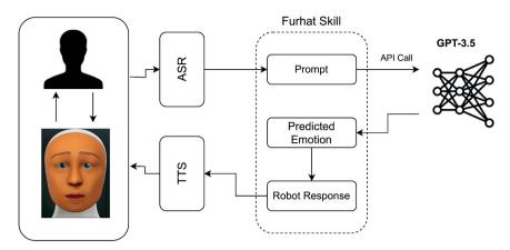
Figure 4.1: Outline of the model used in this study to generate emotions using GPT-3.5
