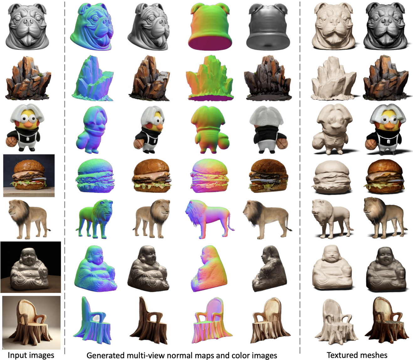
Figure 1. Wonder3D reconstructs highly-detailed textured meshes from a single-view image in only 2 ~ 3 minutes. Wonder3D first generates consistent multi-view normal maps with corresponding color images via a cross-domain diffusion model, and then leverages a novel normal fusion method to achieve fast and high-quality reconstruction.
