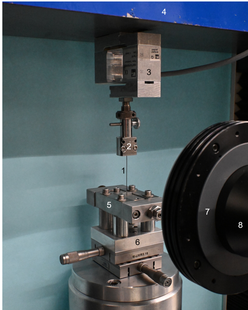
Figure 6.1: Image of the setup used for testing tungsten wires with diameters d \leq 150 \mu\text{m} . Numbers mark the main components of the tensile testing setup: (1) uniaxially stressed wire specimen, (2) upper clamp, (3) load cell, (4) upper (moving) crosshead, (5) lower clamp, (6) x-y-table, (7) ring light, (8) telecentric lens mounted on a CCD camera chip.
