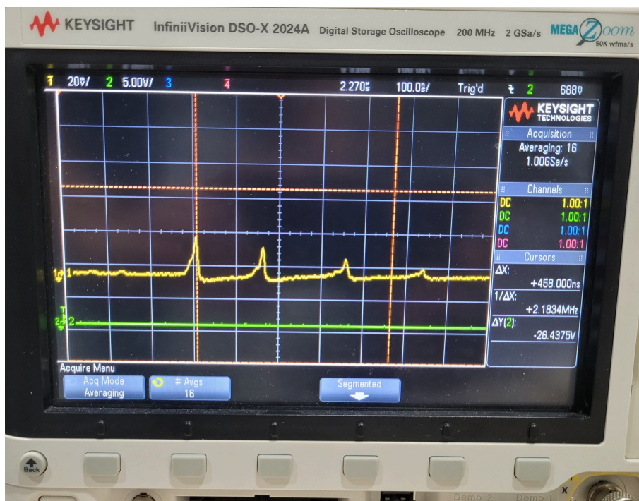
Figure 9: Picture of TOF spectrum displayed on the oscilloscope. Peaks from left to right: C^+ , CH^+ , CH_2^+ , CH_3^+ .
