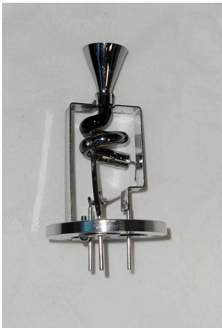
Figure 6: Picture of a channeltron. Ions enter through the conical shape on the top. In the curled metal secondary electrons are emitted. Bottom: the connections for the high voltage.
