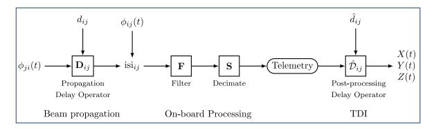
FIG. 1. Flowchart illustrating beam propagation, online and offline processing for the interspacecraft interferometric beatnote phase. The propagation and postprocessing delay are defined in Sec. II and Sec. III B, respectively. Note that the online and offline processing of the reference interferometer, not shown here, is needed to compute the final output of this diagram, the TDI variables.
