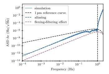
FIG. 7. Commutator residuals from filtering and decimation. We compare the numerically simulated data (solid blue) against analytic models (dashed lines). In dashed blue we show the model for the coupling of the decimation-delay commutator (aliasing) and in dashed red the flexing-filtering effect. For reference we also plot the picometer reference curve in dashed black including the transfer function of the filter.
