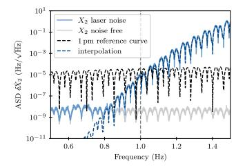
FIG. 4. ASDs of residual laser noise in second-generation Michelson variable  $\dot{X}_2$  due to interpolation errors using Lagrange interpolation with N = 42. The numerical ASD using "atomic" delay operators to perform TDI (solid blue) is compared against the model (dashed blue) and the picometer reference curve (dashed black). The vertical dashed gray line indicates the high frequency edge of the LISA band.
