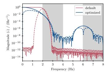
FIG. 6. Magnitude of transfer functions (solid lines) and their frequency derivatives (dashed lines) for the default implementation of the antialiasing filter in LISA INSTRUMENT (red) and the optimized design (blue). The gray and white frequency bands indicate indicate the orientation of the subbands after folding where gray bands are mirrored before they are added to the new band (0 Hz to 2 Hz) and white bands are not.
