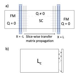
FIG. 8. a) Slice-wise recursive transfer matrix procedure for the ferromagnet-skyrmion crystal-ferromagnet junction. The solid lines highlight the real space discretization and their intersection points are the lattice sites. b) Multiple scattering processes for propagating transmission and reflection matrices. Calculate the transfer matrix for the slab of length  $L_c$ the usual way and then do successive slice wise rotation to propagate the transmission matrices using the infinite series.
