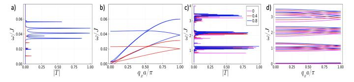
FIG. 9. Transmission and energy spectra for the ferromagnet-skyrmion crystal-ferromagnet junction at normal incidence  $q_y = 0$  at g/J = 0.4 (blue),0.8 (red) and 0 (magenta, only in (c-d)). The effect of increasing g in the 2nd term of the energy functional in Eq. 11 on a) low-energy transmission - peaks shift and increase in height b) Goldstone mode dispersion - modes become more dispersive and c) high energy transmission- slight shift in position of peaks but no significant change in height
