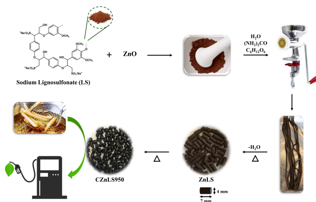
Figure 1. Schematic illustration of synthetic protocol for CZnLS950 using Na-lignosulfonate (LS) and zinc oxide (ZnO) as precursors followed by carbonization at 950 °C, as well as its application as a catalyst for biofuel production from WCO.
