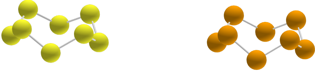
Figure 4.2: Geometries of S_8 (left) of 2.04 Å bond length and Se_8 (right) of bond length 2.33 Å rings structures optimized with HSE06 functional.
