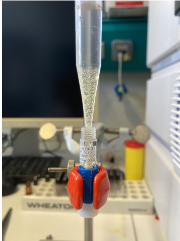
Fig. 3.5: Setup for the packing of AAR in a 25x3 mm BenchMark Microbore column.
