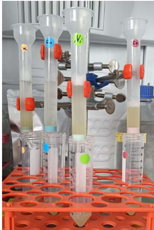
Fig. B.5: Purification of AAR with different resins with the "slurry-method" on gravity-flow columns
