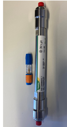
Fig. 3.6: packed EFBR in comparison to a 150x10 mm Chirob T column used for SMB chromatography
