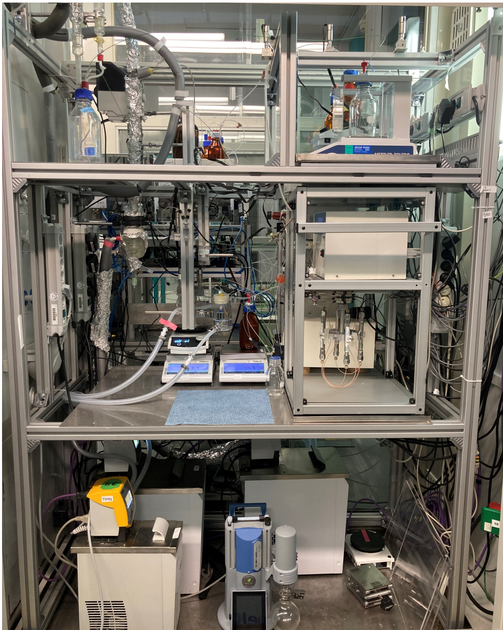
Fig. 3.13: SMB-EFBR-plant. Top: Distillate tank, rectification column, feed and desorbent tank; middle: evaporation tank, EFBR (OA in the back), product tank, SMB unit; bottom: thermostats and evaporation pump.
