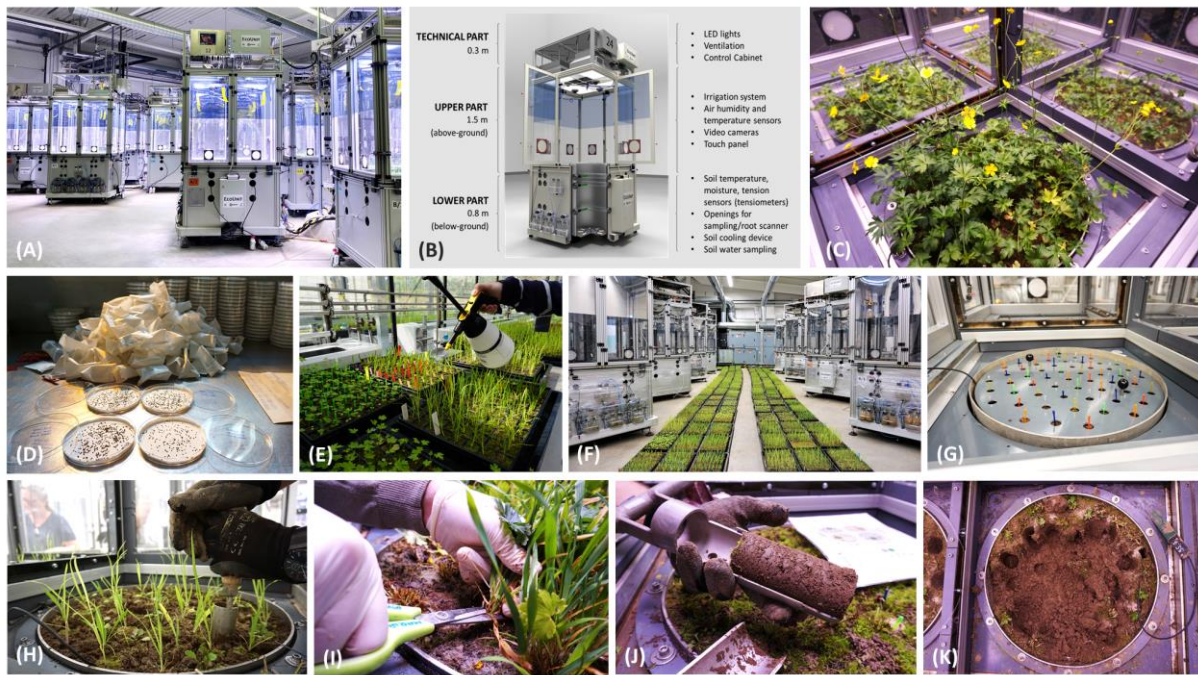
31 Fig. S1. The iDiv Ecotron at the field station of the Helmholtz-Centre for Environmental Research in Bad 32 Lauchstädt, Germany. (A) Photograph of some of the EcoUnits in the Ecotron hall. (B) Schematic depiction of 33 one experimental unit ("EcoUnit") with technical equipment. (C) Photograph of four lysimeters in an EcoUnit 34 with internal walls. (D) Photograph of sowing the seed material in Petri-dishes on filter paper moistened with 35 deionized water. (E) Photograph after pricking plants into plot-specific soil substrate in 96-Quickpot plates. (F) 36 Photograph of all individuals to be planted in the JenaTron Experiment (conducted in 2022) after transport 37 to the iDiv Ecotron. (G) Photograph of the species-specific marking of the positions of all plant individuals on the 38 soil monoliths with the help of a specially-made planting stencil. (H) Photograph of the planting of all plant 39 individuals on the soil monoliths using bulb planters. (I) Photograph of the aboveground plant biomass harvest. (J) 40 Photograph of the soil sampling. (K) Photograph of a destructively sampled lysimeter of the JenaTron Experiment .
