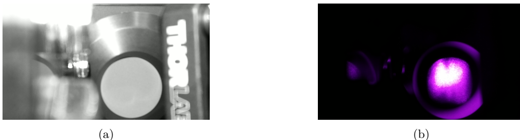
Figure 21: 2 kW laser beam profile on the PM3K in the photodetachment chamber of the CSR. Laser operated in continuous wavemode and 100 ms were selected as exposure time for the camera. a: View of the PM3K with 2 kW laser off and laser box 2 opened. b: View of the PM3K with 2 kW laser turned on and laser box 2 closed.
