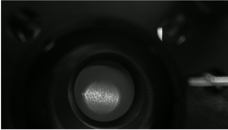
Figure 22: 15 mW laser beam profile on the PM3K in our experiment (experimental setup shown in figure 10) for operation in continuous wavemode and selected exposure time of 25 ms for the camera. The camera is programmed to take grayscale, therefore the 15 mW laser appears grey even though it operates in the visible spectrum.
