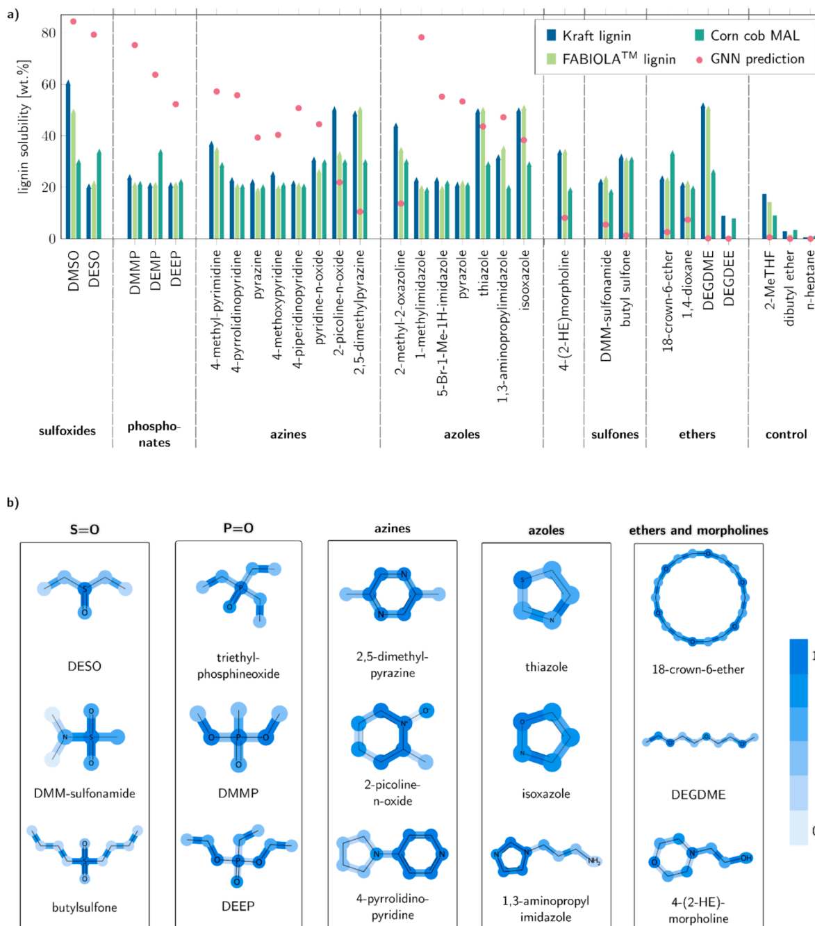
Fig. 4. Experimental validation of the GNN predictions and attribution of structural features to the predicted lignin solubilities. a) Experimental lignin solubilities in the designed solvents for Kraft lignin, FABIOLA TM lignin, and mild acidolysis lignin (MAL) isolated from corn cob. Most solvents were commercially available as originally designed by the genetic algorithm. Otherwise, structurally similar molecules were purchased. Arrows indicate that lignin saturation was not yet reached, however, the high viscosity of the solution hindered measurements with higher lignin loadings. The numerical data is provided in SI. b) Normalised attributions for each discovered solvent class. A higher attribution score of the highlighted structural feature indicates higher importance for the lignin solubility prediction. Abbreviations: DMSO – dimethyl sulfoxide, DESO – diethyl sulfoxide, DMM-sulfonamide – dimethyl methane sulfonamide, DMMP – dimethyl methyl phosphonate, DEMP – diethyl methyl phosphonate, DEEP – diethyl ethyl ethyl phosphonate, 5-Br-1-Me-1H-imidazole – 5-bromo-1-methyl-1H-imidazole, 4-(2-HE)morpholine – 4-(2-hydroxyethyl)morpholine, DEGME – diethylene glycol dimethyl ether, DEGDEE – diethylene glycol diethyl ether, 2-MeTHF – 2-methyl tetrahydrofuran.
