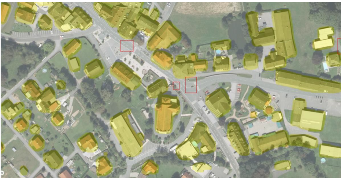
Figure 5. High-resolution aerial image of a part of the rural municipality Heiligenkreuz in the present day. The red bounding boxes mark the automatically detected locations of buildings that featured in the 1820s cadastre. The yellow shade marks the identified present-day buildings.
