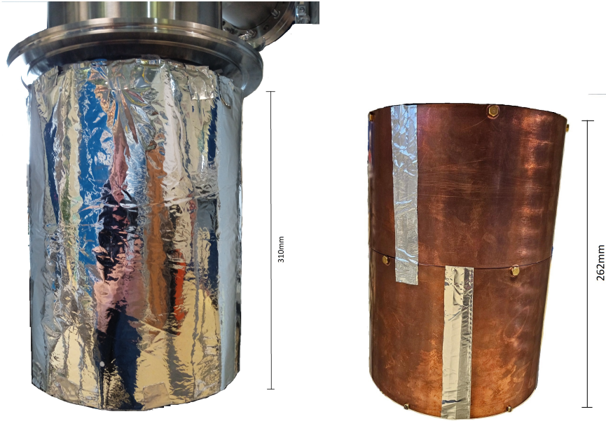
FIGURE 3.4: Left: Aluminum shield with multi layer insulation which is at the 65K stage Right: Copper shield which is at the 4K stage
