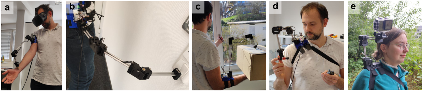
Figure 5: Personalized WRLs offer a broad spectrum of applications, ranging from novel ways of haptic feedback on the body (a) and providing assistance on the go (b) to helping to hold large objects with one hand (c) or tools in peripersonal space (d, e).
