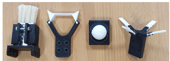
Figure 4: A set of end-effectors: universal fastener, bistable gripper, flexible hemisphere, and 4-legged soft supporter.
