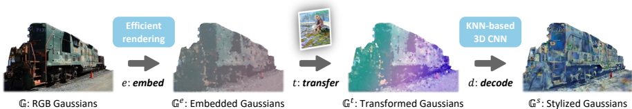
Fig. 2: Overview of StyleGaussian. Given a reconstructed 3D Gaussians \mathbb{G} , we first embed the VGG features to the 3D Gaussians ( e ). Then, given a style image, we transform the features of the embedded Gaussians \mathbb{G}^e to obtain \mathbb{G}^t , where the features are infused with the style information ( t ). Lastly, we decode the transformed features of \mathbb{G}^t into RGB to produce the final stylized 3D Gaussians \mathbb{G}^s ( d ). We design an efficient feature rendering strategy in e that enables rendering high-dimensional VGG features while learning to embed them into \mathbb{G} . We also develop a KNN-based 3D CNN as the decoder in d .
