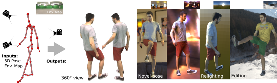
Fig. 1: Our method learns a neural actor that is driven only by a 3D skeletal pose and allows rendering and editing of the actor’s appearance under new lightning and poses not seen during training. Our approach models pose-dependent deformations, self-shadows, and performs intrinsic decomposition of dynamic humans through a pose-dependent mapping between 3D and UV spaces, which also enables editing the appearance and material properties at inference time. For training, our method only needs a multi-view video and an environment map.
