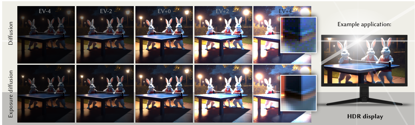
Fig. 1. Existing denoising diffusion models (top row) generate images with low-dynamic range (LDR) on a certain exposure, in the center. When re-exposed to other levels, bright parts like the lamps do not retain their contrast, and dark areas do not reveal details as in the shadow below the table. In our high-dynamic range (HDR) approach (bottom), diffusion is performed at multiple exposures, such that the lamps retain their contrast and the details in the animals’ bodies are produced without noise (see insets). An example application is an HDR display, where high pixel values map to high physical intensity.
