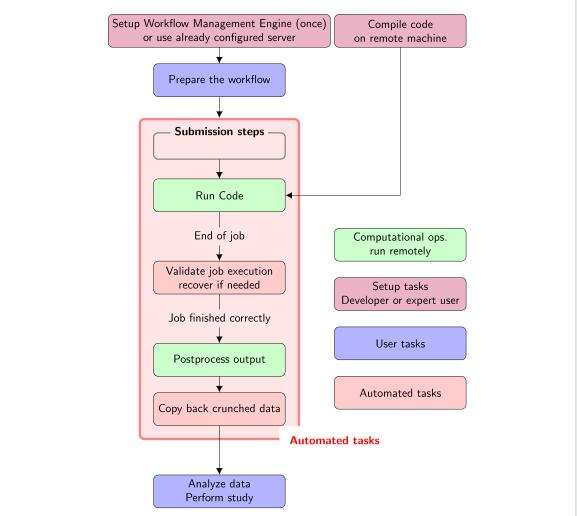
**Figure 4.** Depiction of how a workflow-management engine can be employed for the scheduling of the operations on a remote HPC machine.
