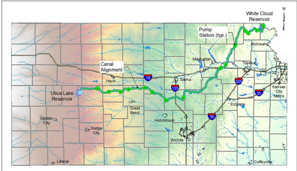
Figure 2. Map of Kansas showing the proposed aqueduct route in green. The aqueduct would begin at the northeastern border of the state, the Missouri River, diverting water from the river near St. Joseph, Missouri, into the yet-to-be-built White Cloud Reservoir in Kansas. From the reservoir, water would travel through 16 pumping stations (green dots) 375 miles (604 km) west via a canal or pipeline to terminal storage in another proposed reservoir in Utica, Kansas. From this second yet-to-be-built reservoir, the water is supposed to recharge the Ogallala/High Plains Aquifer. (Kansas Water Office and U.S. Army Corps of Engineers, 2015: iii).
