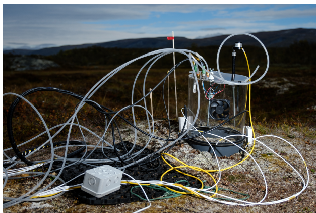
Figure 2. Chamber setup during measurement period, with soil moisture and soil temperature sensors installed in the soil, and all inlets connected. Photo: Fabio Cian
