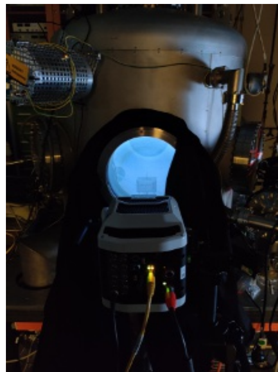
FIG. 1. Picture of the experimental set-up showing the blue argon plasma created by the glow discharge through a vacuum window and the high-speed camera.
