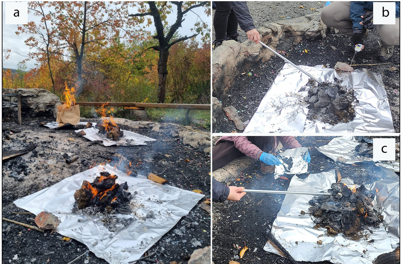
Fig 1. Open fire experiment: a —starting three discrete fires with paper bags full of dry dung, b —temperature recording every 15 minutes, and c —sampling every 15 minutes in an aluminized bag.
