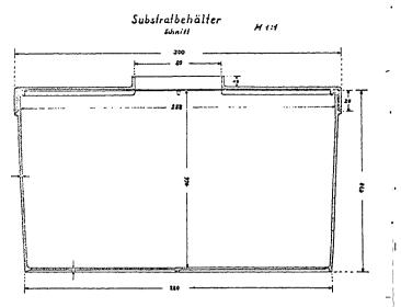
Fig.5 See Fig. 4 Section of the polypropylene container = l0 liters contents: 4 kgs nutritive substrate
