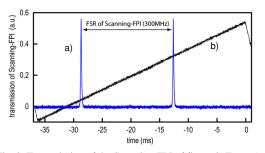
Fig. 3: Transmission of the Scanning-FPI of figure 2. Trace a) shows two successive longitudinal modes of the FPI with no other frequency components in between representing single frequency operation of the high power mode. Trace b) shows the FPI's ramp.
