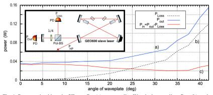
Fig. 1: Power emitted into the SIL arm  $P_{out}$  (a), power split off by the beam splitter  $P_{Loss}$  (b), and power reinjected into the laser  $P_{in}$  (c) plotted as a function of losses in the SIL path. The output power  $P_{HP}$  was nearly constant for all shown waveplate angles. Inset: Corresponding experimental setup.
