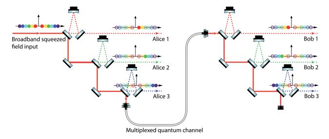
FIG. 4: (Colour online) Distribution of sideband fields of a squeezed field for N=3 EPR channel multiplexing. For each EPR channel a pair of filter cavities and a pair of frequency shifted local oscillators (not shown) are required.
