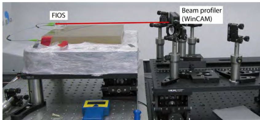
Figure 5.40: Photograph of the set-up for the beam parameter measurement after vibration and shock tests.
