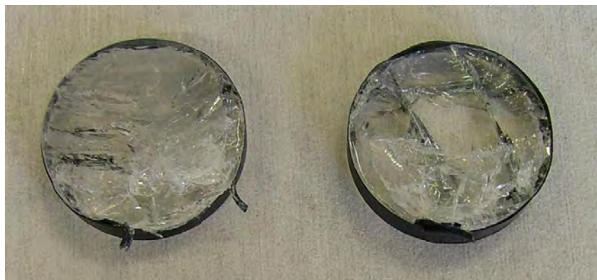
Figure B.18: Photograph of one of the bonded samples after testing.
