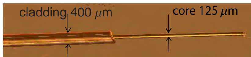
Figure 5.6: Fibre end with removed cladding using dichloromethane; core diameter 125\ \mu\text{m} and cladding 400\ \mu\text{m} .
