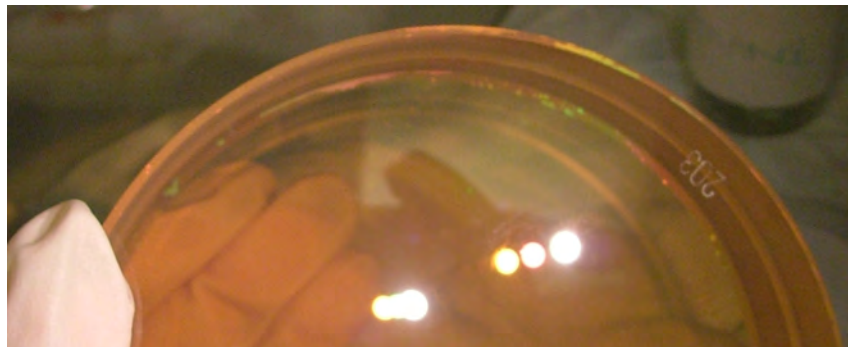
Figure B.14: Photograph of dry areas at the edge of the bond.
