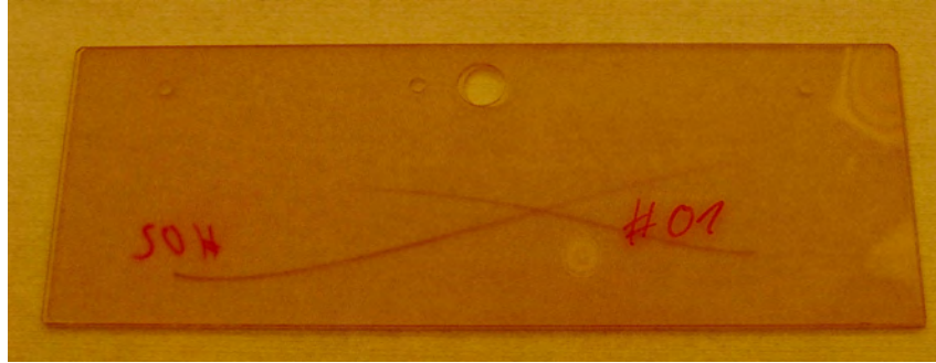
Figure B.10: Photograph of two 100 \times 28 \times 0.8 mm bonded substrate.
