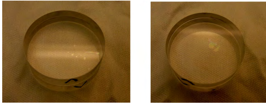
Figure B.15: Photographs of two samples directly after bonding. The rainbow–coloured reflections are indicating air bubbles within the bonded surfaces.
