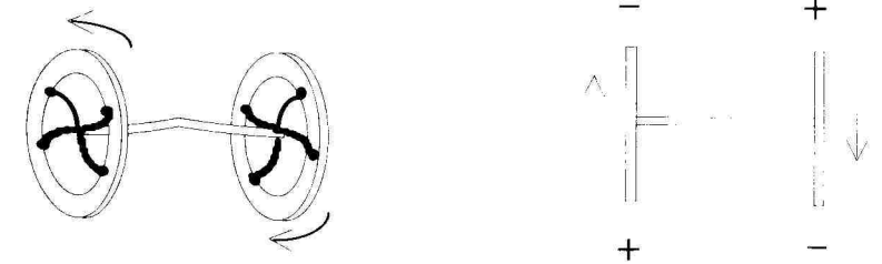
Figure 6.1. A simple current-quadrupole radiator. The left-hand panel shows how the two wheels are connected with blade springs to a central axis. The wheels turn in opposite directions, each oscillating back and forth about its rest position. The right-hand panel shows the side view of the system, and the arrows indicate the motion of the near side of the wheels at the time of viewing. The + signs indicate where the momentum of the mass of the wheel is toward the viewer and the - signs indicate where it is away from the viewer.
