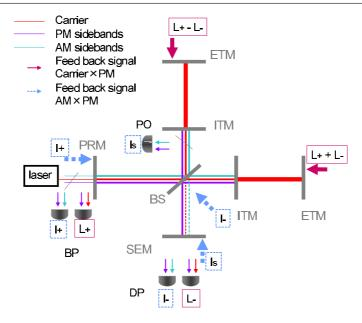
Figure 2. Control of the whole interferometer.
