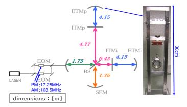
Figure 6. Optical layout of the prototype interferometer.
