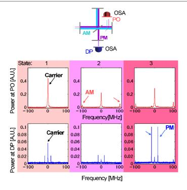
Figure 9. Sideband resonant peaks inside the PRC and the SEC.
