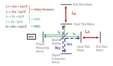
Figure 1. Degrees of freedom in the power recycled RSE interferometer.
