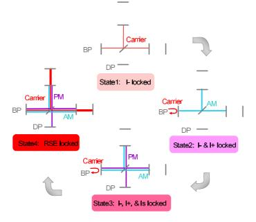
Figure 7. Lock states of the interferometer.
